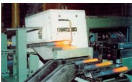
Forging heating is very important process in forging production. The induction heating and heating with gas are the main method in forging industry. How to increase heating efficiency, uniform and temperature accuracy are the vital issues. That large gas furnace with regenerator burning system installed has brought a significant energy saving, and improved the emission, but the energy utilization is still expected to be improved.
